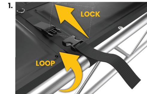
To secure Auroris to ladder truss, loop strap around truss and connect buckles with a click. Ensure the buckle is fully inserted with both prongs locked in place.
